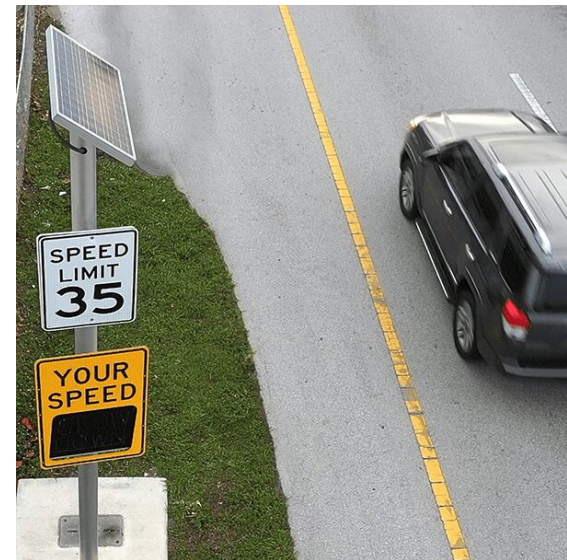
Photo Credit: Carmanah. Example of a smart radar sign.
